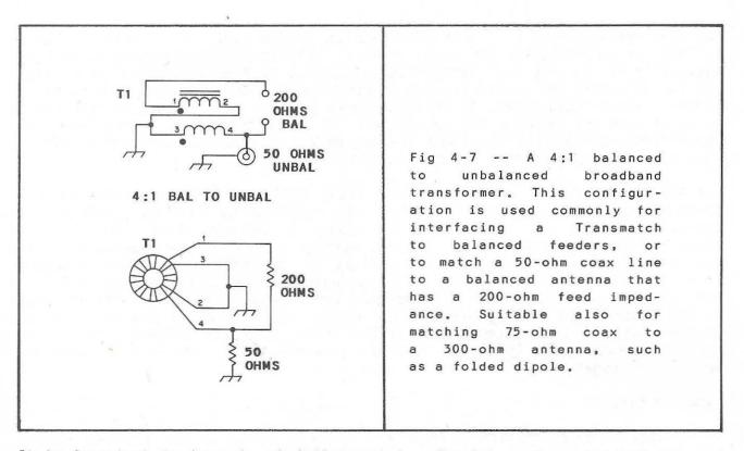
It is important to keep in mind that any broadband transformer should be used in an environment that has load impedances which match the transformation ratio of the transformer. These loads should be resistive rather than reactive in order for the transformer to function correctly. Broadband transformers are intended for use at impedance levels less than 500-600 ohms.
