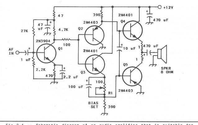
Fig 2-4 -- Schematic diagram of an audio amplifier that is suitable for use in a receiver. Power output is roughly 400 mW. R1 is adjusted for minimum audio distortion while a weak audio signal is applied to the input of the overall amplifier. Copper or aluminum tabs (3/8 X 1 inch) are epoxycemented to the flat sides of Q5 and Q5 to serve as heat sinks. Overall amplifier current drain is 125 mA at peak audio periods.
