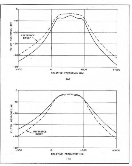
Fig 4—Frequency response of the filter of Fig 2 with changes in the end terminations. Curve A shows response with 150-ohm terminations; curve B shows the response using 300-ohm resistors. See the text for considerations of which is "better."
