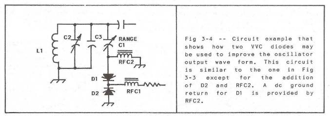
Since D1 and D2 of Fig 3-4 are in series, the net capacitance will be half that of one diode. You may select diodes that have twice the capacitance required for the desired tuning range. The correct amount of effective capacitance will then be available when the diodes are connected as in Fig 3-4.
