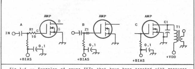
Fig 1-4 -- Examples of power FETs that have been treated with measures to suppress or damp VHF oscillations. A 10-ohm resistor is used at the gate of Q1 at A. This R1 component should be located as close to the transistor as practicable. A ferrite bead (Z1) is used for this purpose at B. A drain bypass capacitor (C1) damps VHF oscillations at C. Its XC should be four times or greater the transistor drain impedance to prevent signal loss.
