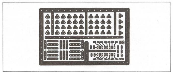
Fig 4-3 -- Scale etching pattern for a universal breadboard. This W1FB design includes a + voltage bus at the center of the pattern. Various ground foils come from the outer perimeter of the board to permit short leads for grounded components. A 16-pin DIP IC site is at the lower right. No. 60 holes are drilled in the copper pads to facilitate parts installation.
