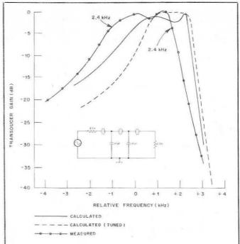
Fig. 9 — Measured and calculated (with and without tuning) results for a wider bandwidth filter for use in a simple ssb exciter. Crystals are the same as used for the filter of Fig. 8.
