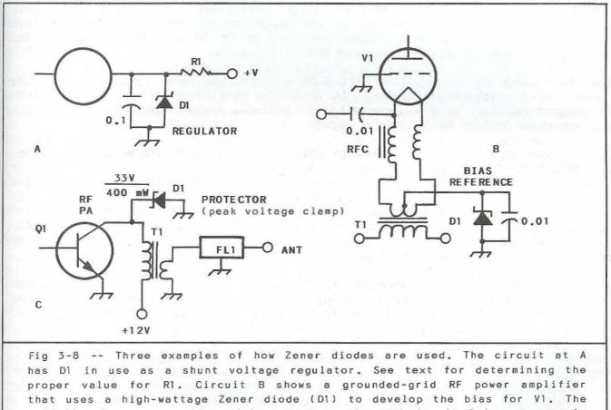
grid thus becomes negative with respect to the cathode. At C is an example of how to use a Zener diode to protect Q1 from high SWR or voltage peaks that can occur during periods of self-oscillation. D1 also protects against voltage spikes that may occur on the dc supply line.
