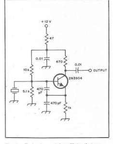
Fig. 4 — A simple crystal oscillator that may be used for crystal frequency matching. The 470-pF capacitors may be ceramic, mica or polystyrene. This circuit will function with crystals from 1.8 MHz to over 10 MHz.
