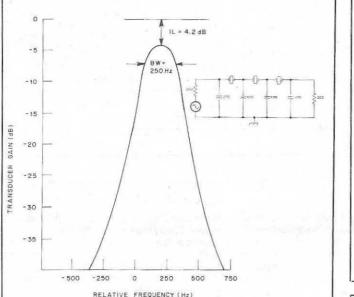
Fig. 6 - Circuit and calculated response for a 3-pole crystal filter at 3.577 MHz with a 250-Hz bandwidth. The design is based on measurements on surplus TV color-burst crystals.
