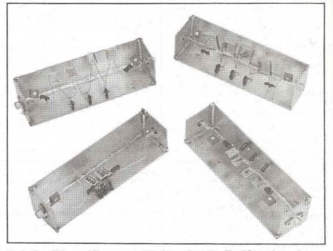
Fig A—Four CW crystal filters were built in this configuration. The PC-board mounting surfaces provide a ground plane. Capacitors are soldered directly to the ground plane, and the crystals are connected using the capacitors as standoffs. Phono jacks are used for input and output connectors. The only variables in the construction of the filters are the crystal characteristics and the length of the crystal leads. The SSB filter is not shown.
