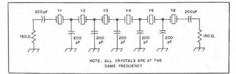
Fig 5-Circuit of a Cohn filter using six crystals.
