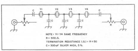
Fig B—Schematic diagram of the crystal filters. Capacitors are all of equal value. Terminating resistors are variable 500-ohm units. Crystals are all of equal nominal frequency with minor (up to 50-Hz) variation.
