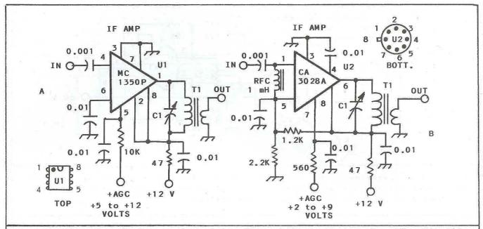
Fig 3-14 -- Practical examples of two IF amplifiers that employ ICs. Circuit A contains a low-cost Motorola MC1350P. AGC control voltage is +5 to +12, with maximum amplifier gain at +5 V. C1 and T1 in both examples are tuned to the IF. Approximate input Z for both circuits is 1K ohms. Output impedance is on the order of 4K ohms. Circuit B uses an RCA CA3028A IC. AGC voltage for this device is +2 to +9, with maximum gain occurring at +9 V. Both amplifiers can provide up to 40 dB of gain.
