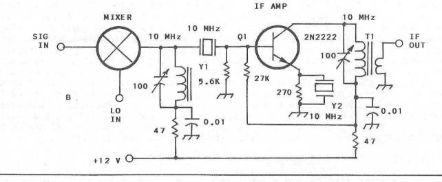
Fig 5-8 -- Circuit A shows 455-kHz IF transformers connected as an LC IF filter that is suitable for AM or SSB reception. Circuit B utilizes two-low-cost computer crystals to provide IF selectivity (see text).
