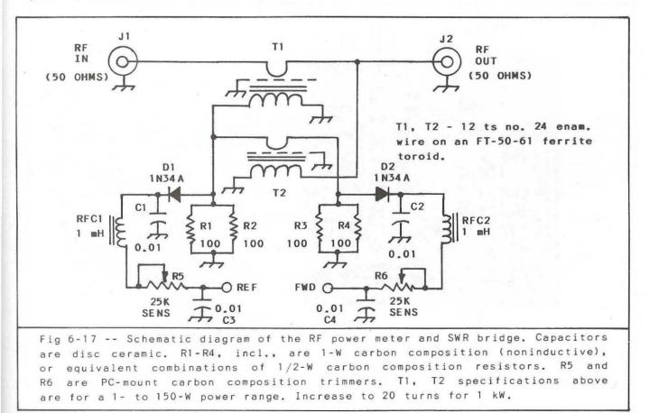
You may use silicon diodes, such as 1N914s, for D1 and D2 in Fig 6-17 if you build the bridge for power levels above 100 W. It is preferable to use germanium diodes for QRP power measurements. This is because they conduct at lower voltage levels than is characteristic of silicon diodes. This effect can result in no meter reading when the reflected power is low, which suggests the SWR is 1 when it may be 1.5:1 or greater.
