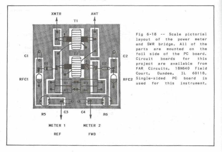
The circuit board in Fig 6-18 need not be so large. The layout can be compressed to provide a much smaller instrument. Wide conductors are desirable in order to minimize stray inductance. I made my prototype PC board by removing the unwanted copper with a hobby motor and small cone-shaped abrasive bit. Strips of thin copper may be glued to a piece of Formica or similar insulating material in lieu of a standard PC board.
