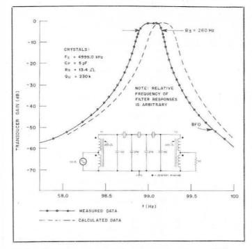
Fig. 8 — Comparison of calculated and measured results on a 5-MHz cw filter. The crystals had  $\rm F_{o}$  = 4.999 MHz,  $\rm C_{p}$  = 5 pF,  $\rm R_{s}$  = 13.4 ohm and  $\rm Q_{u}$  = 230,000. A proper BFO frequency is marked. See text for discussion.
