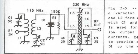
Fig 3-5 -- Practical example of a varactor frequency doubler. L1 and L2 form a bandpass tuned circuit with C1 and C2. A resonant cavity is used for C3 and L4 to provide low output for unwanted harmonic currents. C4 and C5 are adjusted to provide an impedance match from D1 to the output load (50 ohms).
