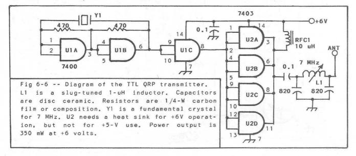
I want to stress that I have not tried the circuit in Fig 6-6. Were I to put it on the air I would definitely add a harmonic filter after the pi network. I presume that the circuit can be keyed by breaking the +6-V lead to pin 14 of U1. You may wish to key the U1 pin 7 lead instead. Certainly, this little transmitter could be used nicely as a miniature emergency rig for hikers and campers.
