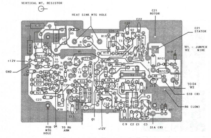
Fig 6-14 -- Enlarged X-ray view of the PC board for the 40-meter transceiver as viewed from the component side of the board. W1 may be omitted if both **b** abd **g** are connected to J4. The black band indicated the cathode end of the diodes. The electrolytic capacitors should be installed in accordance with the polarity shown.
