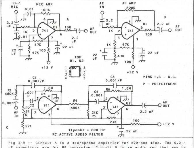
uF capacitors are for RF bypassing. Circuit B is an audio amp that may be used as a preamp or as the output stage of a receiver that uses head phones. A two-pole RC active CW filter is shown at C. Numbered resistors are 5% types. C1 through C4 should be closely matched in value.
