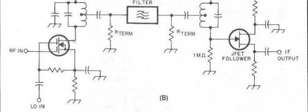
as those at 3.579 MHz. While an SSB filter can be built at 3.579 MHz, probably higher terminating impedances will be required. The termination value drops with increasing frequency, making wider bandwidth filters more easily realized at higher frequencies. I often build equipment with a 10-MHz IF because crystals with excellent Q are readily available for this frequency.
