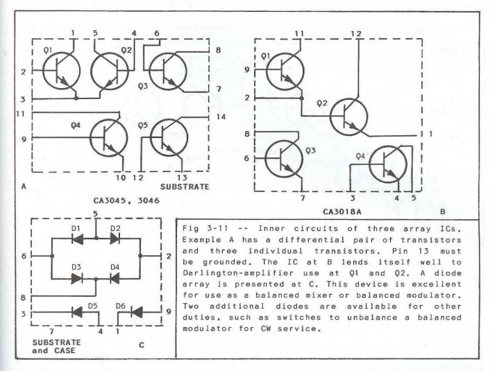
modulator. The inner workings of the aforementioned ICs are shown in Fig 3-11.
