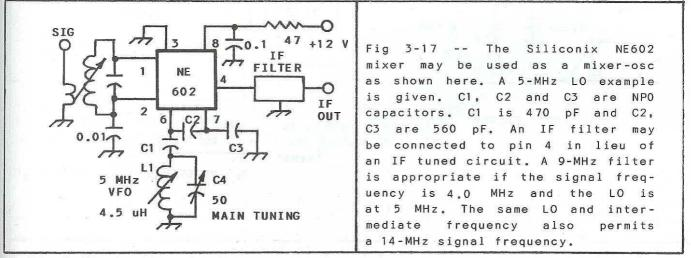
In Fig 3-17 pin 6 is the base of the internal oscillator transistor and pin 7 is the emitter. The circuit above is for a Colpitts oscillator. This use of the NE-602 is ideal when we wish to build simple DC and superheterodyne receivers. It is better to use an outboard LO with buffering for high-performance receivers. Oscillator harmonics can cause performance problems when the LO transistor is on the same substrate as the remainder of the IC circuitry.
