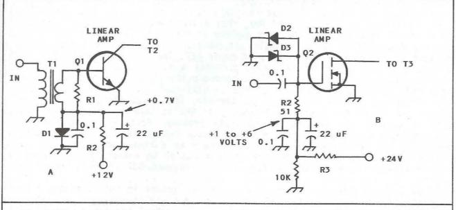
application of forward (positive) bias to the base of the BJT and the gate of the power FET.
