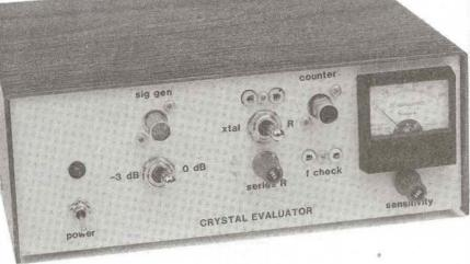
indications of the crystal characteristics. Q1 provides a 50- $\Omega$  load for the output of the crystal.
