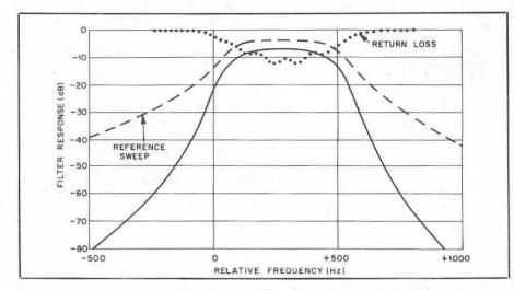
Fig 6—Frequency response of the six-crystal filter. The reference sweep is the response of the three-crystal filter of Fig 2.
