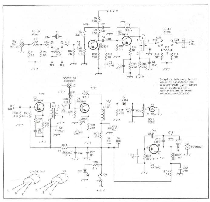
Fig 1—Schematic diagram of the RF portion of the crystal tester. Capacitors are disc ceramic, 100 V. Those with polarity marked are electrolytic or tantalum. Fixed-value resistors are ¼-W carbon composition.
