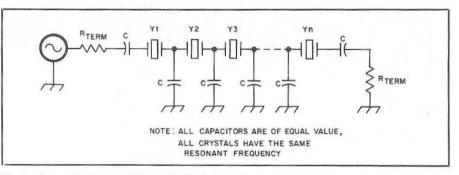
Fig 1-Generalized crystal filter suitable for empirical construction.
