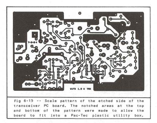
The PC board in Fig 6-15 is available as a drilled and plated item from FAR Circuits, 18N640 Field Court, Dundee, IL 60118. I do not recommend that you attempt to build this project on the universal PC board described earlier in this book. Perf Board or "ugly construction" is not recommended either.
