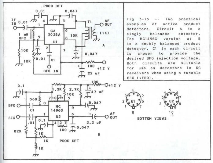
Fig 3-15A show how to use the familiar RCA CA3028A as a singly balanced PD. T1 is a miniature audio transformer with a 10K-ohm center-tapped primary and a 1K-ohm secondary. The bypass capacitors at pins 3 and 8 can be chosen to provide a bandpass audio response with the primary inductance of T1. These capacitors also help to roll off high-frequency response and reduce audio hiss. BFO input voltage should be on the order of 1 to 1.5 V RMS.
