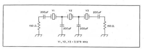
Fig 2-A simple CW filter using three crystals.
