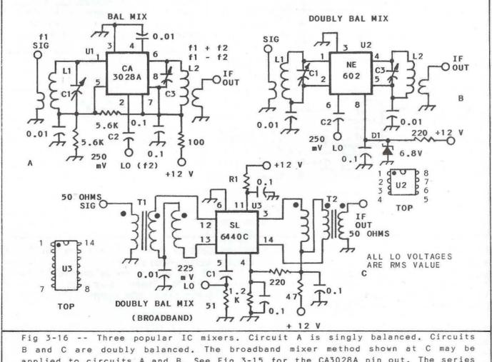
B and C are doubly balanced. The broadband mixer method shown at C may be applied to circuits A and B. See Fig 3-15 for the CA3028A pin out. The series capacitor at each IC LO pin is chosen to establish the mV injection value listed, which should appear at the related IC pin.
