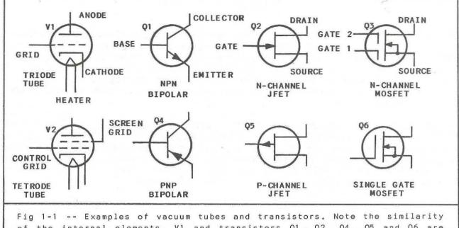
of the internal elements. V1 and transistors Q1, Q2, Q4, Q5 and Q6 are triode (three element) devices. V2 and Q3 are similar. Q3 could be called a tetrode if it has a cathode. The NPN devices require a positive operating voltage on their collectors, while PNP transistors must have a negative collector voltage (emitters connected to ground). N-channel FETS use a plus voltage on their drains, while P-channel FETs require a minus drain voltage.
