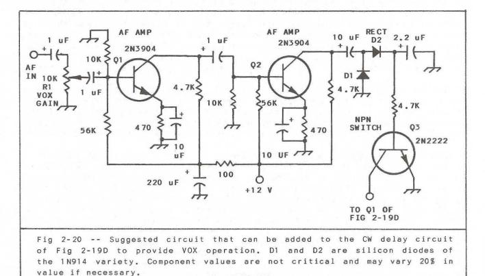
Input for this circuit is obtained from the mic audio line or from the output of one of the speech-amplifier stages in the SSB transmitter. R1 is adjusted to ensure VOX actuation at normal speech levels and operator distance from the
