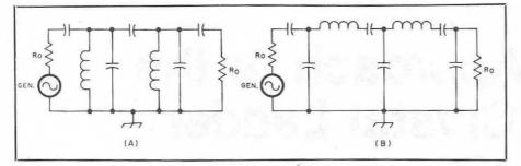
Fig. 1 — Double-tuned circuits with equal termination at each end. Parallel resonators are used at A; series-tuned circuits are used at B.
