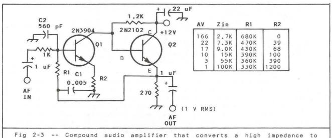
a low impedance. Suitable for use with a high-Z mic and a low-Z transceiver mic input, C1 is chosen to roll off the high-frequency audio response. C2 is an RF bypass capacitor. The chart shows various amplifier gains and input impedances that result from selected resistor values.
